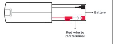
Then slide the battery in fully and replace the cover.
