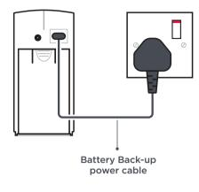
The ONT **Power** light should be on or flashing to indicate it is working. The battery takes 24 hours to become fully charged and the ONT can still be used in the meantime.
